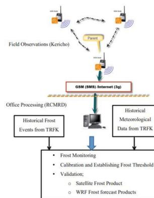
Figure 6: Wireless Sensor Network configuration
