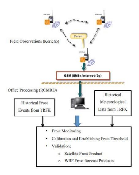
Figure 6: Wireless Sensor Network configuration
