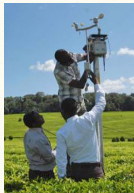
RCMRD has installed a Wireless Sensor Network at Tea Research Institute for validation of satellite data
