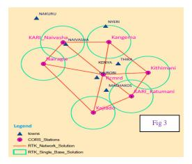
Stations at spans of at most 70-80km from RCMRD shall form the basic network. The idea is to have 360 degrees RTK Network solutions coverage within Nairobi and 30km RTK single base from each station beyond the network solutions limits.
