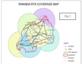
The new stations proposed are located at Kibungo, Nyagatare, Busogo, Ruharambuga and Butare. It's also proposed that the new station where possible be collocated within Automatic Weather Station (AWS)sites (yellow symbols in fig 2 above)
